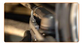
Tighten the tie rod end locknut. Use a combination spanner #23. Use a combination spanner #24. Use a torque wrench. Tighten it to 50 nm torque.
