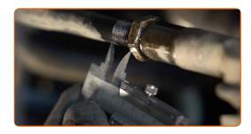
Loosen the lock nut securing the tie rod end to the tie rod. Use a combination spanner #24.
