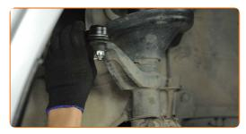
Tighten the tie rod end locknut. Use a combination spanner #24. Use a torque wrench. Tighten it to 50 nm torque.
