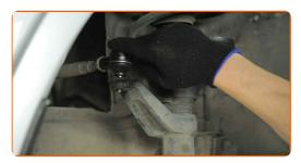
Tighten the fastening nut connecting the tie rod end to the steering knuckle. Use a combination spanner #19. Use a torque wrench. Tighten it to 43 nm torque.
