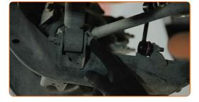
Unscrew the lower fastener of the shock absorber strut. Use a drive socket #17. Use a tap wrench. Use a ratchet wrench.
