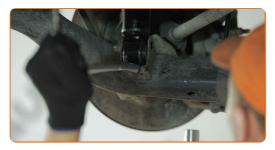
Install the fastening bolt. Use a crowbar. Use a drive socket #17. Use a ratchet wrench.
