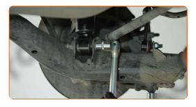
Remove the support from under the arm.
