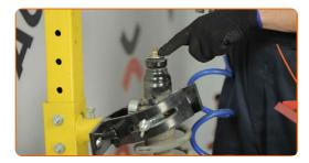
Remove the strut piston rod nut. Use a combination spanner #17. Use HEX No.H6. Use a ratchet wrench.
