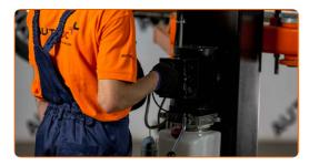
Attach the bottom part of the shock strut. Use a crowbar. Use a flat screwdriver.
