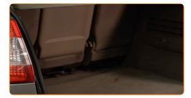
Remove the side plastic cover. Use a flat screwdriver.
