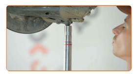
Tighten the lower fastening of the shock absorber. Use a drive socket #17. Use a torque wrench. Tighten it to 93 nm torque.
