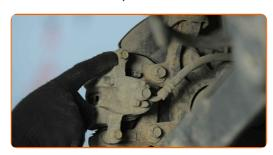
Unscrew the brake caliper fastening. Use a combination spanner #17. Use a drive socket #12. Use a ratchet wrench.
