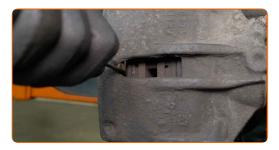
Remove the brake caliper. Use a crowbar.
