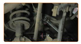
Install the rod fastening to the stabilizer and tighten it. Use a combination spanner #17. Use a drive socket #17. Use HEX No.H6. Use a torque wrench. Tighten it to 38 Nm torque.
