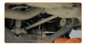
Unscrew the fastener connecting the stabilizer link to the stabilizer bar. Use a combination spanner #14. Use a drive socket #14. Use a ratchet wrench.
