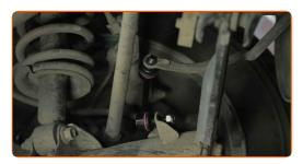
Tighten the fastener connecting the stabilizer link to the stabilizer bar. Use a combination spanner #17. Use HEX No.H6. Use a torque wrench. Tighten it to 38 Nm torque.
