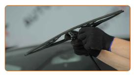
Remove the blade from the wiper arm.
