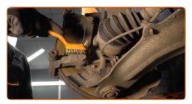
Unscrew the caliper bracket fastening. Use a drive socket #17. Use a ratchet wrench.
