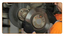
Clean the hub. Use a wire brush. Treat the contacting surface. Use copper grease.
