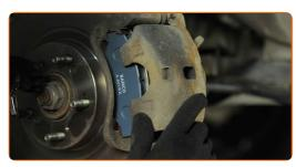
Use a drive socket #12. Use a torque wrench. Tighten it to 34 Nm torque.
