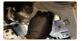
Screw in the new drainage plug and tighten it. Use a drive socket #17. Use a torque wrench. Tighten it to 39 nm torque.
