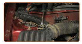
Detach the engine wiring harness.
