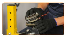
Tighten the shock strut piston rod nut. Use a drive socket #19. Use a torque wrench. Tighten it to 55 Nm torque.
