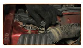
Unscrew the fasteners of the engine wiring harness bracket. Use a drive socket #10. Use a ratchet wrench.
