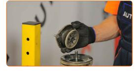
Release the coil spring.
