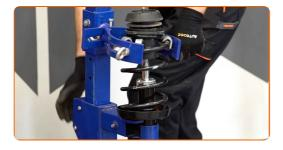
Remove the assembled shock strut.
