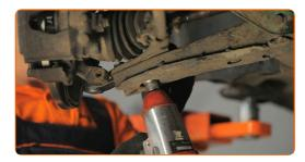
Connect the ball joint to the steering knuckle. Use a crowbar. Use a rubber mallet.
