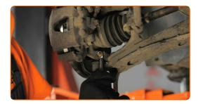
Remove the fastening bolt. Use a hammer.
