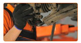
Tighten the ball joint fastener. Use a combination spanner #18. Use a drive socket #18. Use a torque wrench. Tighten it to 55 nm torque.
