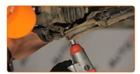
Release the fastener connecting the ball joint to the steering knuckle. Use a flat metal-working chisel. Use a hammer.
