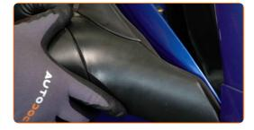
Tighten the screws of the wing mirror. Use a drive socket #8. Use a torque wrench. Tighten it to 8 Nm torque.
