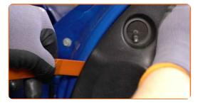
Remove the wing mirror screws. Use a drive socket #8. Use a ratchet wrench.
