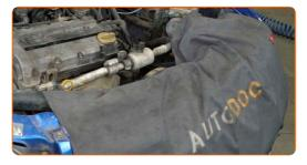
Detach the connector from the ignition coil.
