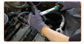
Treat the ignition coil connector with electronic spray. The spray will protect the electrical contacts from corrosion, oxidation, and will reduce the contact resistance.
