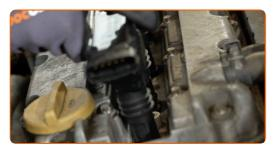
Tighten the ignition coil bolts. Use Torx T30. Use a torque wrench. Tighten it to 8 nm torque.
