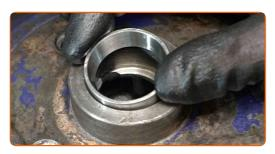
Install the new inner race of the wheel bearing into the brake drum. Bush and bearing driver set.
