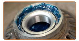
22 Install the wheel bearing oil seal.
