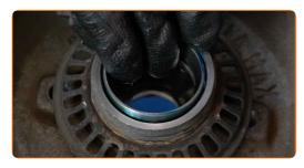
Treat the wheel hub bearing. Use bearing grease.
