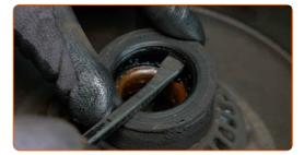
Remove the wheel hub bearing. Use a crowbar.
