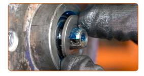
Screw on the hub nut. Use a drive socket #24. Use a ratchet wrench.
