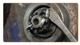
Unscrew the hub nut. Use a drive socket #24. Use a ratchet wrench.
