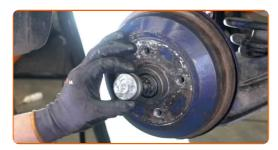
Remove the cotter pin securing the hub nut. Use a crowbar. Use a flat screwdriver.
