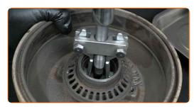
Remove the wheel bearing's outer race from the brake drum. Use a bush and bearing driver set.
