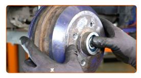
Fit the wheel bearing washer.
