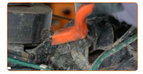
Unscrew the lower fastener of the shock absorber. Use a drive socket #17.
