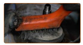
Loosen the upper fastener of the shock absorber. Use a combination spanner #14. Use a shock absorber socket DDNº5,2.
