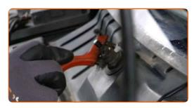
Unscrew the plastic panel fasteners. Use a combination spanner #24.
