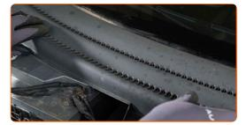
Install and secure the cowl grille. Use a drive socket #8. Use a ratchet wrench. Use a Phillips screwdriver.
