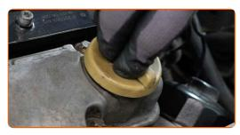
Tighten the oil filler cap.
