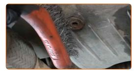
Unscrew the drain plug. Use HEX No.H7. Use a ratchet wrench.
