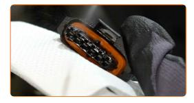
Plug in the ignition coil connector.
