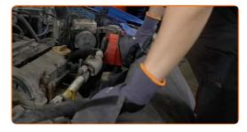
Detach the connector from the ignition coil.
