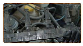
6 Clean dirt, dust and debris from inside the spark plug wells.
