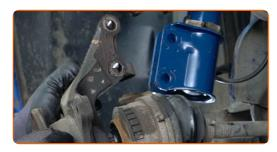
Detach the driveshaft from the steering knuckle.
