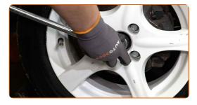
Tighten the drive shaft nut. Use a drive socket #30. Use a torque wrench. Tighten it to 20 Nm torque.+90°
