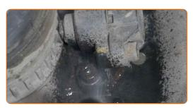
Unscrew the ABS sensor fastener. Use HEX No.H5. Use a ratchet wrench.
