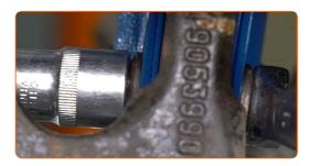
71 Fit the wheel bearing washer.
