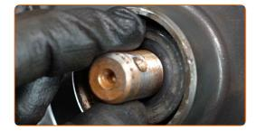
Screw the nut of the drive shaft. Use a drive socket #30. Use a ratchet wrench.
