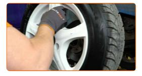
Unscrew the fastener connecting the drive shaft to the wheel hub. Use a drive socket #30. Use a ratchet wrench.
