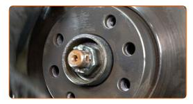
75 Tighten the brake disc fastening. Use a Phillips screwdriver. Use a torque wrench. Tighten it to 7 Nm torque.
