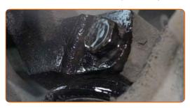
Unscrew the ball joint fastening to the steering knuckle. Use a combination spanner #13. Use a drive socket #13. Use a ratchet wrench.
