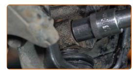
Screw in the fastener that connects the shock strut to the steering knuckle. Use a combination spanner #18. Use a drive socket #18. Use a ratchet wrench.
