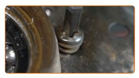
Remove the brake disc cover.
