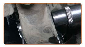
Remove the fastening bolt.
