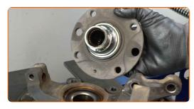
Clean the wheel hub bearing retaining ring.
