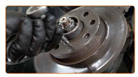
76 Install the brake caliper bracket.
