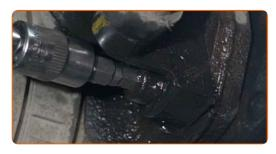
Remove the fastening bolt.
