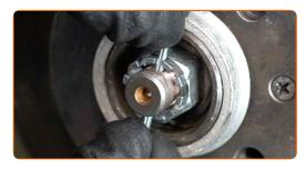
92 Install the cap of the hub nut. Use a rubber mallet.
