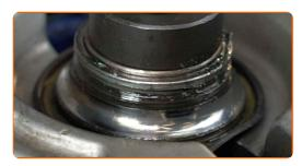
Clean the hub bearing mounting seat. Use a wire brush. Use WD-40 spray. Use all-purpose cleaning spray.
