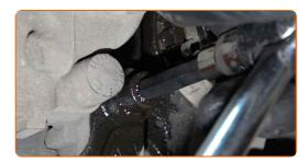
20 Remove the brake caliper together with its bracket.
