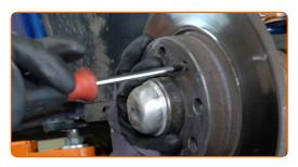
18 Remove the brake disc.
