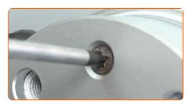
Tighten the brake disc fastening. Use a Phillips screwdriver. Use a torque wrench. Tighten it to 7 Nm torque.
