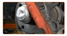
20 Install the brake disc.
