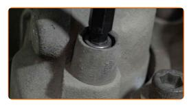
Remove the brake caliper.
