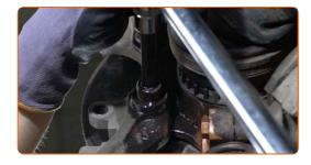
Remove the caliper bracket.
