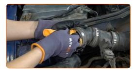
6 Release the air filter cover clips.
