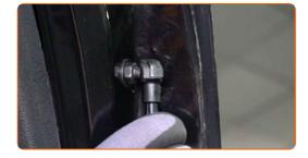
Release the circlip connecting the gas strut to the boot lid. Use a flat screwdriver.
