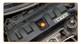
Screw in the engine cover fasteners. Use a flat screwdriver.
