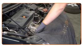
Unscrew the engine cover fasteners. Use a flat screwdriver.
