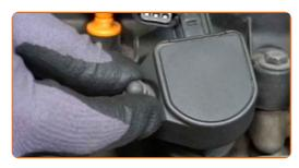
Tighten the ignition coil fasteners. Use a drive socket #10. Use a torque wrench. Tighten it to 9 nm torque.
