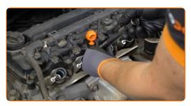
Screw new spark plugs and tighten them. Use the spark plug socket #16. Use a torque wrench. Tighten it to 23 nm torque.
