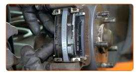
21 Install the brake caliper and fasten it.
