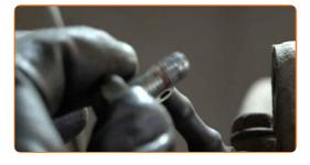
Remove the brake caliper.
