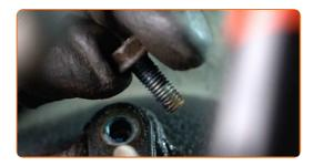
Remove the ABS sensor. Use long nose pliers.
