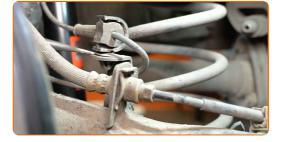
Clean the ABS sensor connector. Use a nylon cleaning brush.
