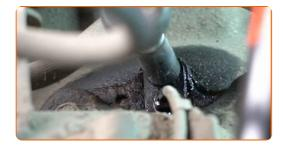
11 Remove the fastening bolt.
