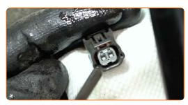
Treat the mounting seat of the ABS sensor. Use a multipurpose grease.
