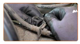
Attach the ABS sensor connector.
