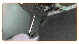
Install and secure the cover under the glove box.
