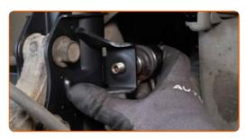
Tighten the fastener connecting the stabilizer link to the shock strut. Use a drive socket #17. Use a torque wrench. Tighten it to 30 Nm torque.
