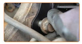
Tighten the lower fasteners connecting the shock strut to the steering knuckle. Use a combination spanner #19. Use a drive socket #19. Use a torque wrench. Tighten it to 106 Nm torque.
