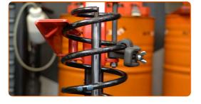
Install the dust boot and the bump stop on the new shock absorber.
