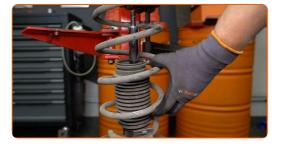
Remove the old shock absorber from the hydraulic coil spring compressor.
