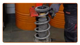
Remove the shock absorber dust boot and bump stop.
