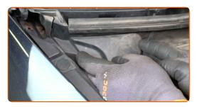
Remove the cap from the suspension strut mount.
