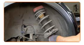
Clean the mounting seats of the shock strut. Use a wire brush.
