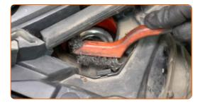
6 Loosen the upper fasteners of the suspension strut. Use a drive socket #14. Use a ratchet wrench.
