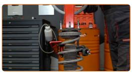
Unscrew the strut piston rod nut. Use a 19-mm strut nut socket. Use HEX No.H6. Use a ratchet wrench.
