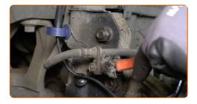
Unscrew the fastener that connects the brake hose bracket to the suspension strut. Use a drive socket #12. Use a ratchet wrench.
