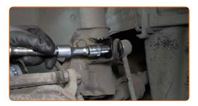
Unscrew the fastener connecting the stabilizer link to the stabilizer bar. Use a drive socket #14. Use a ratchet wrench.
