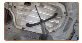
Unscrew the oil pan guard fasteners. Use a drive socket #10. Use a ratchet wrench.
