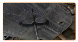
7 Unscrew the engine splash guard fasteners. Use a drive socket #10. Use a ratchet wrench.
