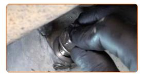
Reinstall the engine oil drain plug and tighten it. Use a drive socket #17. Use a torque wrench. Tighten it to 30 Nm torque.
