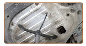
Screw in the oil pan guard fasteners. Use a drive socket #10. Use a ratchet wrench.
