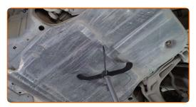
Tighten the engine splash guard fasteners. Use a drive socket #10. Use a ratchet wrench.
