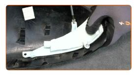
Treat the connector of the turn signal repeater light. Use dielectric grease.
