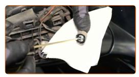
Attach the connector of the turn signal repeater light.
