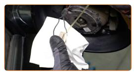
19 Attach the mirror heating connectors.
