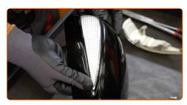
Screw in the fasteners connecting the turn signal repeater light to the mirror cover. Use Torx T20.
