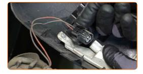
Unscrew the fasteners of the turn signal repeater light from the mirror cover. Use Torx T20.
