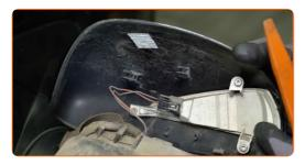
Detach the connector of the turn signal repeater light.
