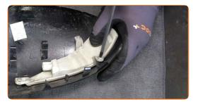
Remove the turn signal repeater light.
