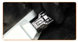
Install the wing mirror housing. Make sure you hear a click indicating that it is locked in place.
