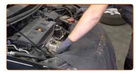
Release the air filter cover clips.
