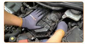
11 Press the air filter cover clips into place.
