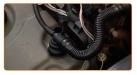
5 Remove the crankcase ventilation hoses.
