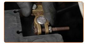
Screw in the negative battery terminal fastener. Use a combination spanner #10.
