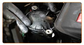
Tighten the fasteners of the fuel filter housing cover. Use HEX No.H4. Use a torque wrench. Tighten it to 9 Nm torque.
