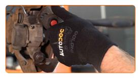
14 Remove the brake caliper.
