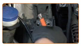
Treat the engine mount fasteners. Use a sealant.
