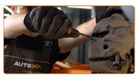
10 Remove the brake caliper.
