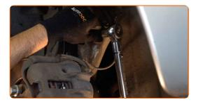
Tighten the fastener connecting the stabilizer link to the stabilizer bar. Use a drive socket #17. Use a torque wrench. Tighten it to 40 Nm torque.
