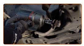
Unscrew the fastener connecting the stabilizer link to the shock strut. Use a drive socket #17.
