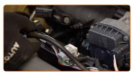
Disconnect the crankcase ventilation hose from the intake manifold.
