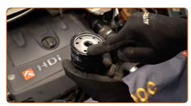
Screw the new filter into its place. Use the 74/76-15F socket. Use a torque wrench. Tighten it to 25 Nm torque.
