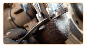
Remove the brake pads. Use a crowbar.
