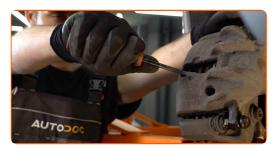
10 Remove the brake caliper.
