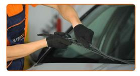
Remove the blade from the wiper arm.
