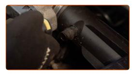
Detach the throttle valve connectors.
