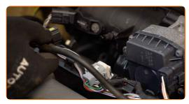
Disconnect the crankcase ventilation hose from the intake manifold.
