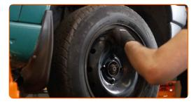
Unscrew and remove the wheel arch cover fasteners. Use a clip removal tool. Use a Phillips screwdriver.
