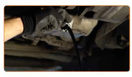
Replacement: engine oil and filter – CITROËN Xsara Box Body / Hatchback (N3\_). Professionals recommend:
