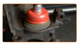
Press the new bearing in the steering knuckle. Bush and bearing driver set.
