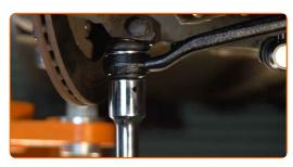
Tighten the front fastener connecting the control arm to the subframe. Use a drive socket #18. Use a torque wrench. Tighten it to 74 nm torque.
