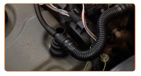
5 Remove the crankcase ventilation hoses.
