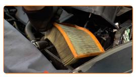
Cover the air intake hose with a microfibre towel to prevent dust and dirt from getting into the system.
