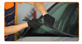
Remove the blade from the wiper arm.
